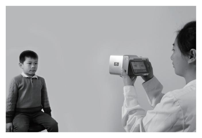
The Cell vision screener V100 is a portable diagnostic device designed for clinicians to quickly detect vision abnormalities on patients from 6-month old to adults. Cell can screen both eyes at once from a distance of 1 meter. Once the pupils are in focus, the device will start to calculate automatically and deliver results within 1 second. The touch screen allows users to operate conveniently like using a smart phone.
